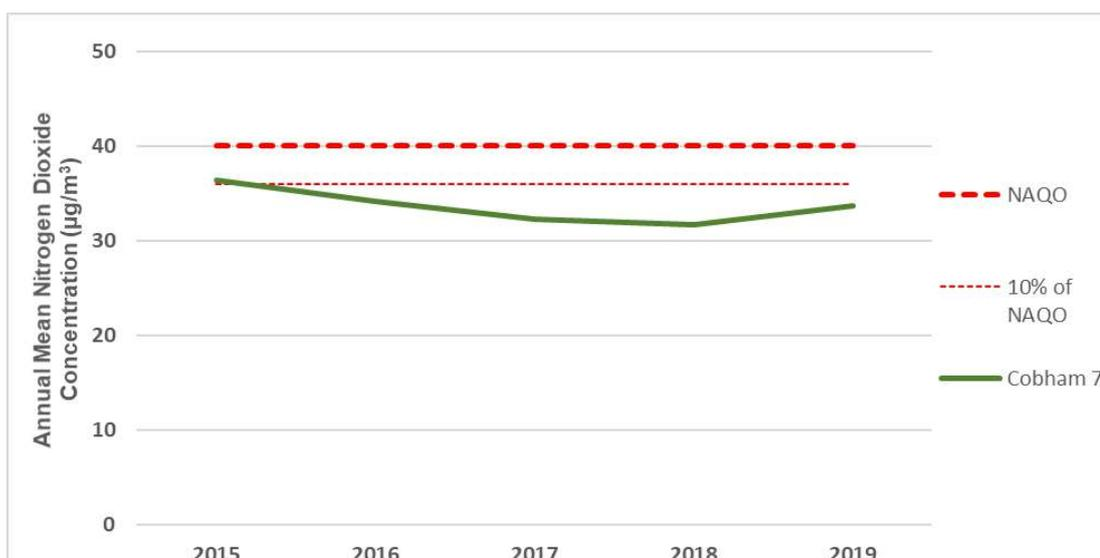
Figure 4.2: Trends in Annual Mean NO<sub>2</sub> Concentrations at the Cobham 7 Monitoring Site
