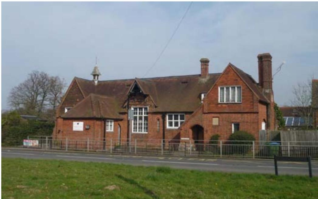
Figure 22: The Old School House to the north was constructed c1880s and has distinct elements of the domestic revival with its steep tile hung gables, bellcote and arched openings in brick
