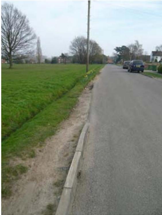
Figure 12: The absence of kerbs adds to the rural character of the area but has led to erosion of the Common edge in places
